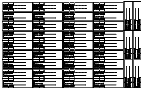
Drawing Three:Lay 1 bundles in each layer.Install in 3 layers.7 bundles,42 tubes in all. (圖3)每層放2捆。分3層放入,側邊豎起放一捆,一盒共7捆,共42管) Disposing schematic diagram of Tube in the inner box, for reference. (管在內盒的擺放示意圖,供參考)
